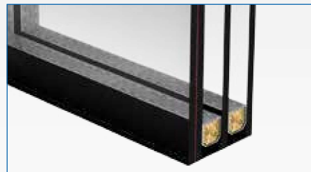
3-glass packet 44.4/14/4/14/4 SECURITY AND PROTECTION
