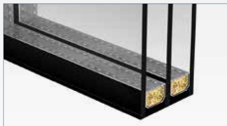
3-glass packet 4/18/4/18/4 WARMTH AND EXTRA LIGHTING
